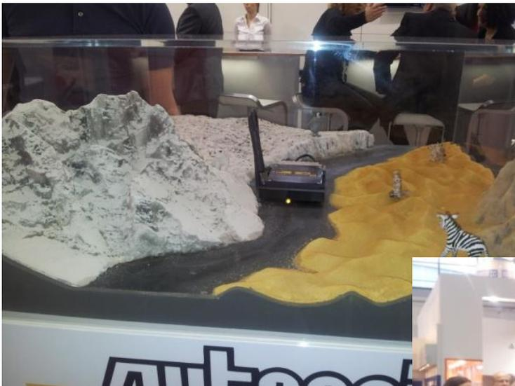
A modeled landscape demonstrated the EMC strength of our converters. We have discharged a 30-40kV voltage to the converter directly, generated by a coil. The status LED showed that it did not impress the converter.
